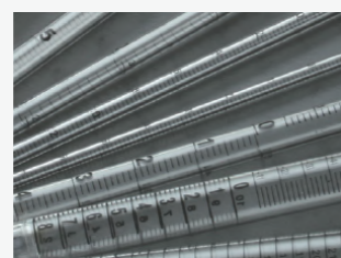
Designed with dual graduation markings, ensuring the pipet volume can be easily identified
