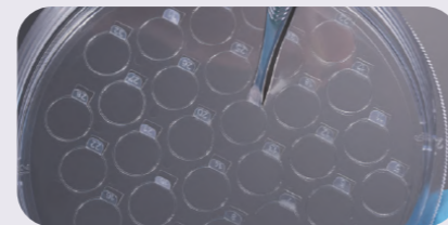
The handle of coverslip is tilted at a certain angle so that operators could hold them easily.
